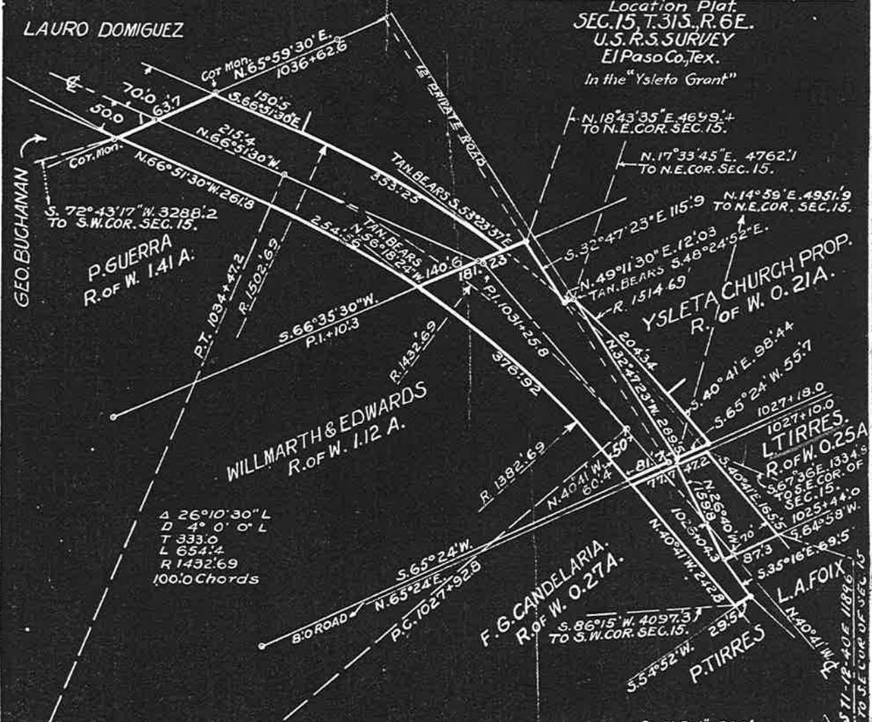
Note: Curve lengths based on 100.0 Chord lengths.
